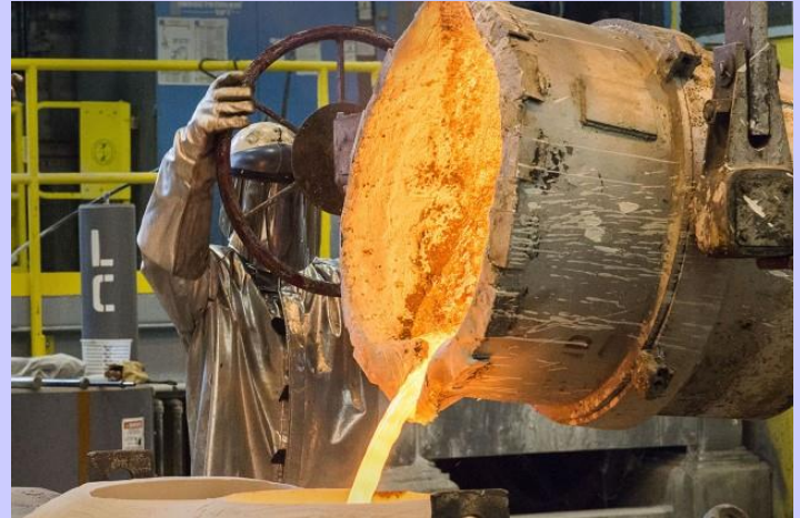
A ladle operated by Marc Morotini (A572) containing liquid molten brass is tipped to fill the mold in the Foundry. Photo by John Whalen
