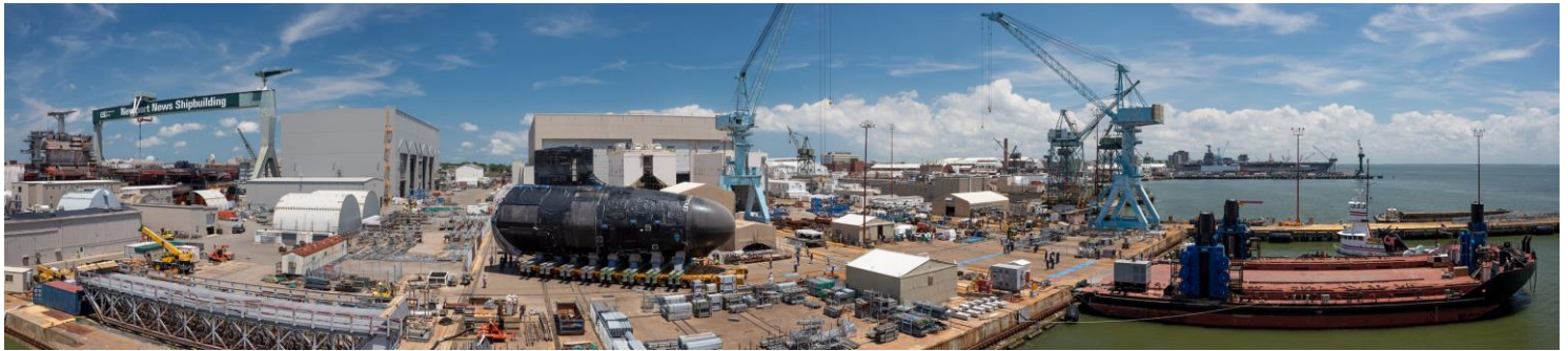
A panorama of Newport News Shipbuilding taken from the Floating Dry Dock showing the bow unit of submarine Illinois (SSN 786) being moved to the sea shuttle. Photo by Chris Oxley
