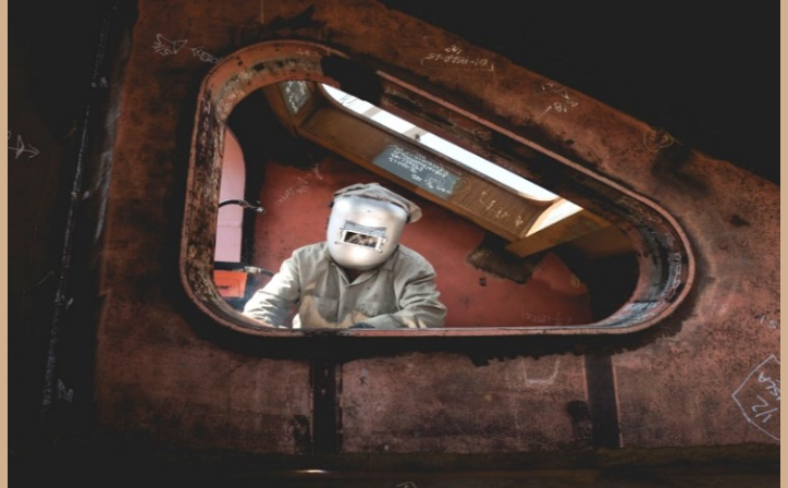
Tommy Morse is framed by a coaming on a John F Kennedy CVN 79 unit as he performs welding operations. Photo by Matt Hildreth.
