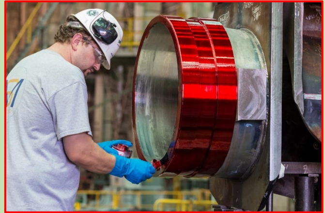
Dye Penetration Test on a South Dakota (SSN790) torpedo tube shutter door. Photo by Chris Oxley
