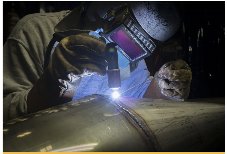
Shipbuilder Tom Forrest performs a precise weld to join aluminum pieces together. Photo by Matt Hildreth
