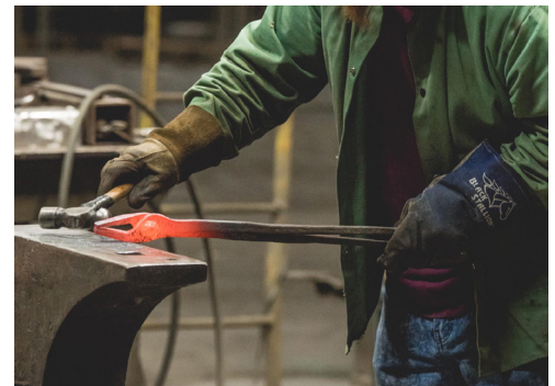
Newport News Shipbuilding’s sole blacksmith, Justin Fitzhugh , shapes a red hot tool in his forge in the Foundry. Photo by Ashley Cowan
