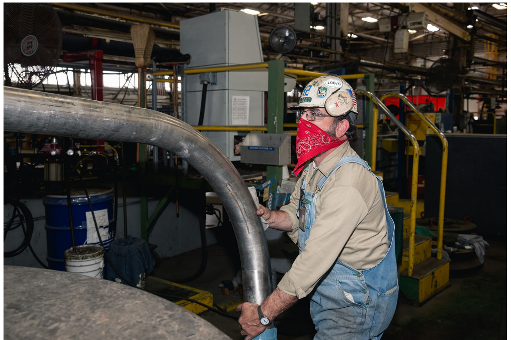
C.L. Gilbert maneuvers a pipe in a bending machine. Photo by Matt Hildreth
