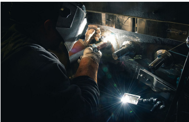
Matthew Peters performs welding operations on the hull of Virginia -class submarine Montana (SSN 794). Photo by Matt Hildreth
