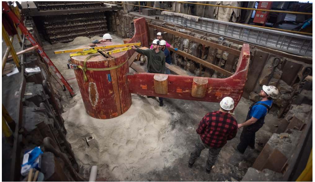
Shipbuilders use a pattern from CVN 65 to create a mold for CVN 80. Photo by Matt Hildreth
