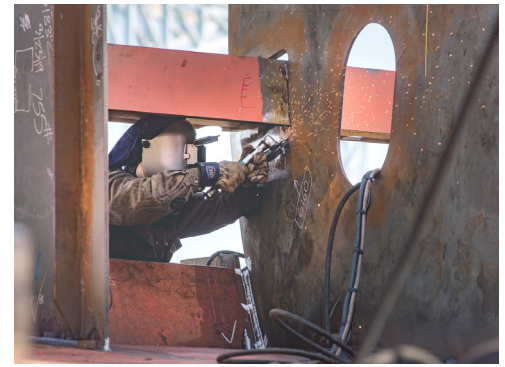
A shipbuilder grinds on an Enterprise (CVN 80) unit located on Platen 21. Photo by Ashley Cowan
