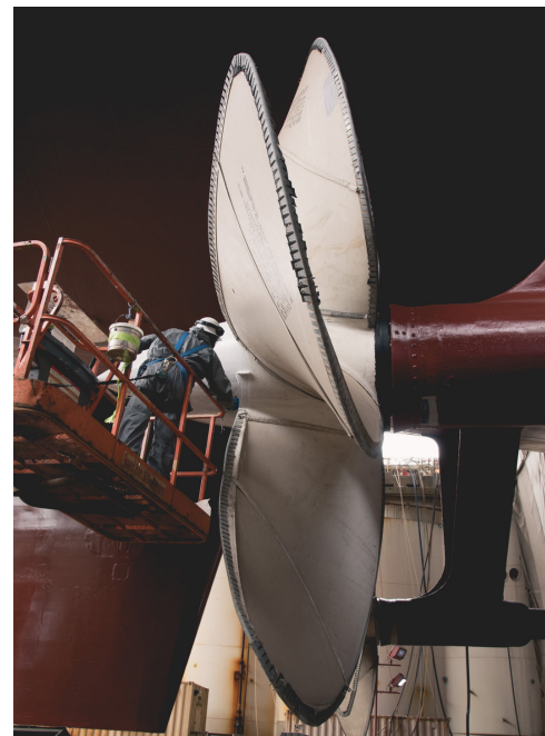
Larry Shoulars touches up one of USS George Washington's (CVN 73) propellers during the ship's refueling and complex overhaul. Photo by Ashley Cowan
