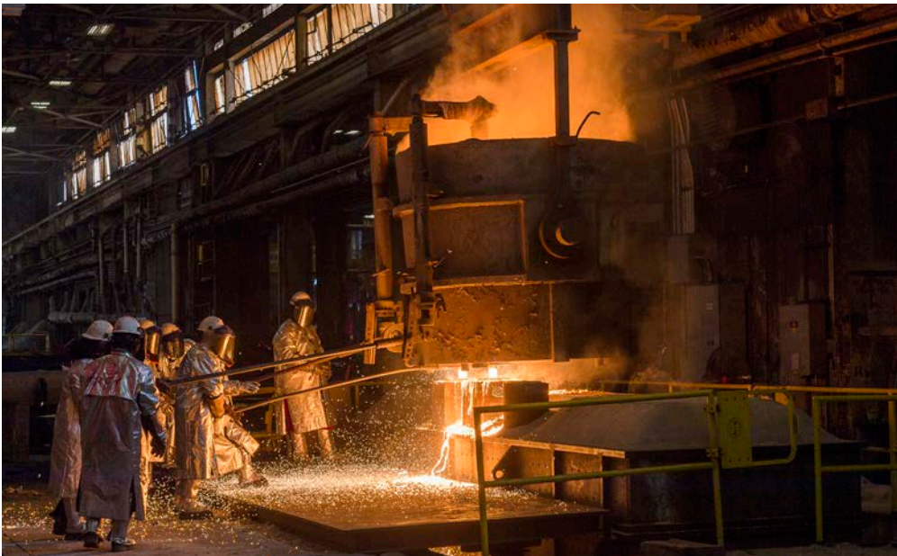
The Foundry team begins the pour for a John F. Kennedy (CVN79) steel elevator guide rail. Photo by John Whalen
