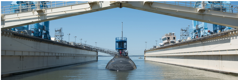
Shipbuilders flood the Floating Dry Dock with USS Washington (SSN 787) inside. Photo by Ashley Cowan
