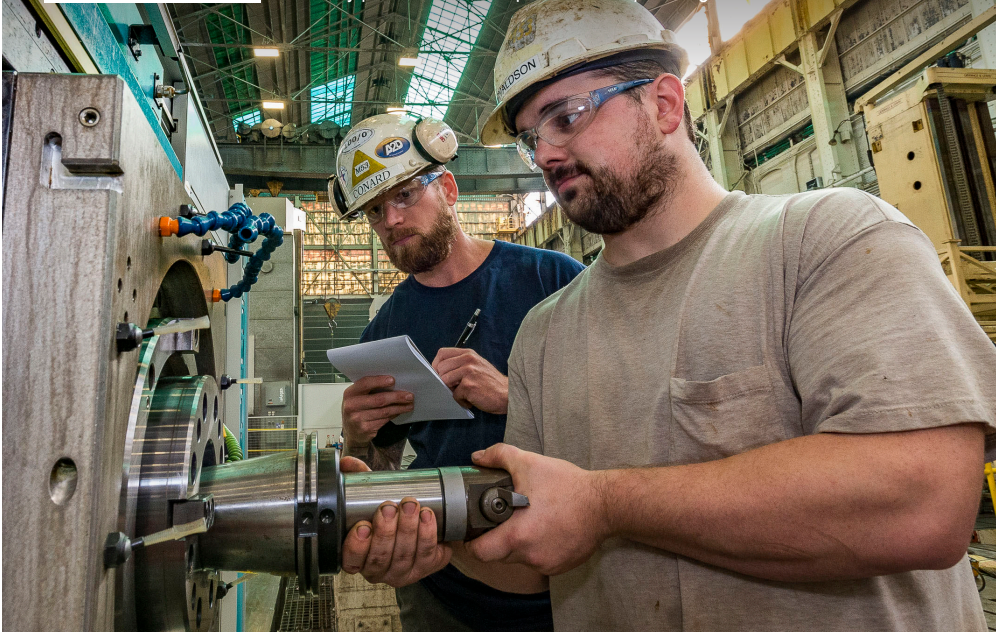
Foreman Brett Conard , left, watches as Eric Thorvaldson Jr. changes a tool on the computer numerical control (CNC) horizontal machining center in the Machine Shop. Photo by John Whalen
