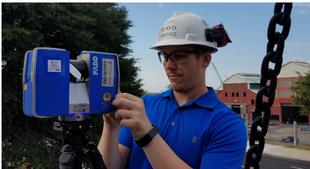
Designer Sean Harris adjusts the FARO laser scanner aboard Dorothy .
