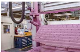
Cover Photo: Chris Perry operates the Pattern Shop's five-axis CNC machine as it cuts a shape out of foam. Photo by John Whalen
