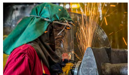
Kenneth Hamilton (A572) grinds the surface of newly cast steel, honing the shape to precise specifications. Photo by John Whalen
