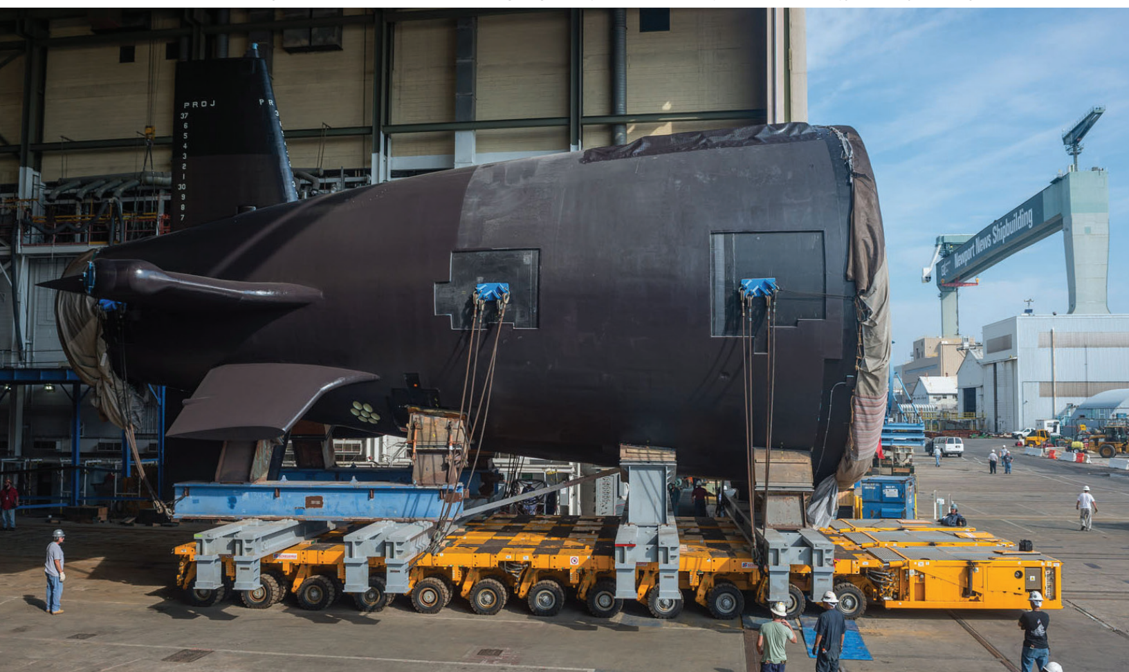
▼ The stern unit of South Dakota (SSN 790) begins the move to the Sea Shuttle. Visit nns.huntingtoningalls.com/photos to view additional photos from around the shipyard. Photo by Chris Oxley
