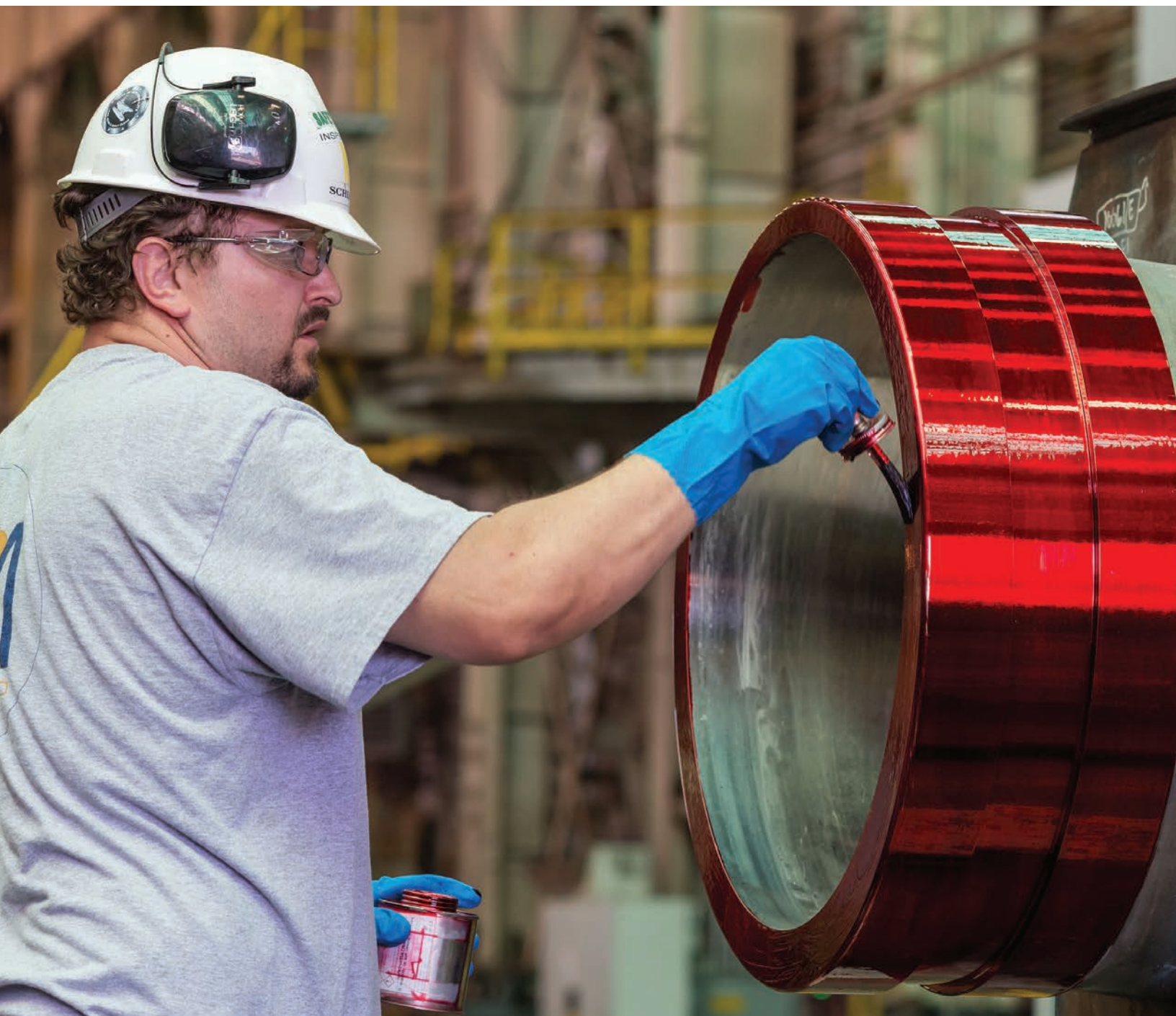
▼ John Schiavone applies the dye for a Dye Penetration Test on a South Dakota (SSN 790) torpedo tube shutter door. Photo by Chris Oxley
