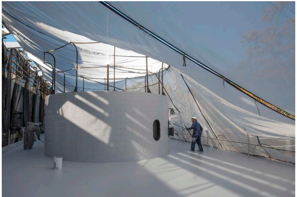
O43 Painters Lee Womble and Rudolph Taylor Jr. paint a second primer on the turret of the replica USS Monitor , which is on exhibit at The Mariners' Museum. Photo by John Whalen
